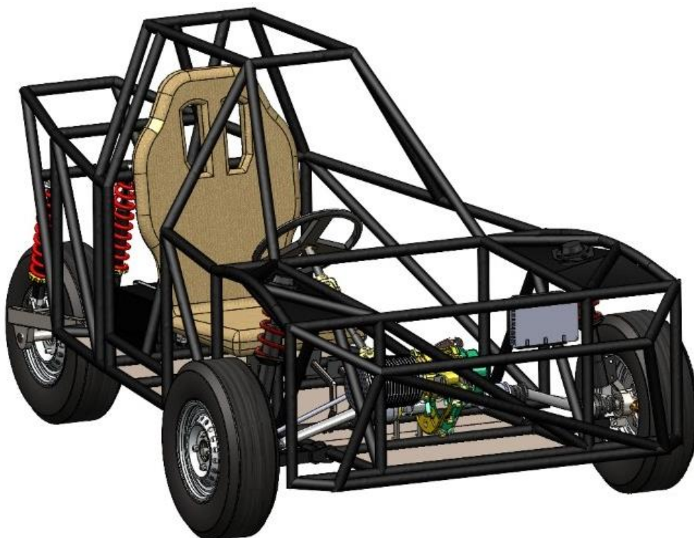
Fig 8.02: Assembly of Tadpole vehicle using Solidworks
